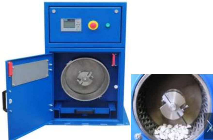
Fig.5. Bond Abrasion Index (Ai) Tester
