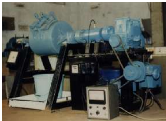
Fig.7. Ball Mill Work Index Unit
