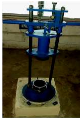
Fig.2.Impact crusher for drop weight tests
