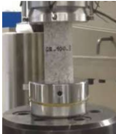
Fig.1.Unconfined Compressive Strength Test of Rock
