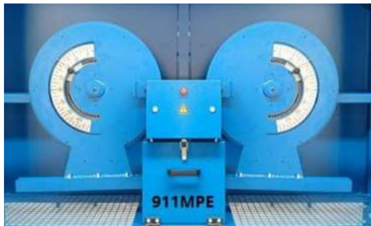
Fig.4. Bond Impact Crushing Work Index unit [by the impact of twin pendulums]
